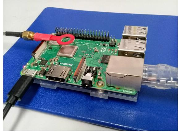
**Figure 1:** Setup for recording EM radiation [5]
