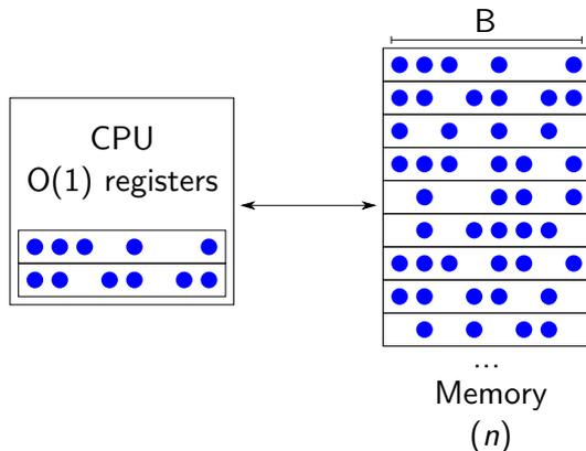
Figure 4: Floyd’s idealized two-level storage. With a fixed number of registers in CPU and the main memory of size  $n$  being split to blocks of size  $B$ .
