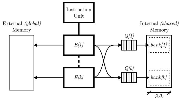
Figure 16: The K-model architecture consisting of  $k$  PEs, an instruction unit, queued internal memory and the external memory.
