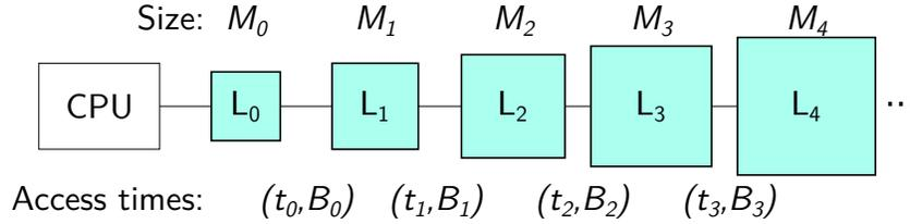
Figure 7: The Memory Hierarchy models cache sizes, block sizes and access times of all the memory levels in the hierarchy.
