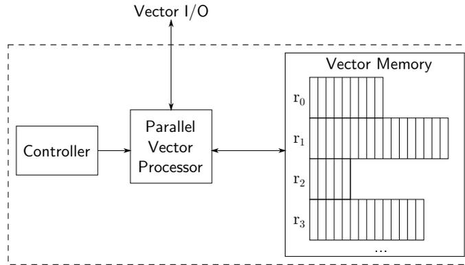
Figure 15: Vector RAM architecture consisting of the Controller, Vector CPU and Vector memory consisting of arbitrarily large vector words. The scalar memory and scalar CPU can also be present separately, but are omitted in the figure.
