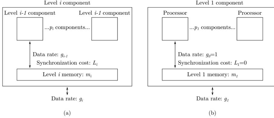
Figure 10: a) Schematic diagram of the Multi-BSP model component structure for the level  $i$ . b) Level 1 component.
