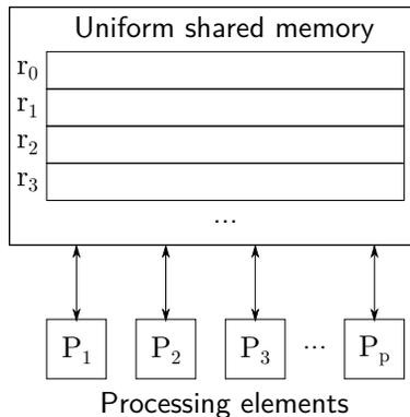
Figure 9: The PRAM model consisting of  $p$  processing elements and a uniform shared memory. Processors' local private memory, accumulator and program counter register are omitted.
