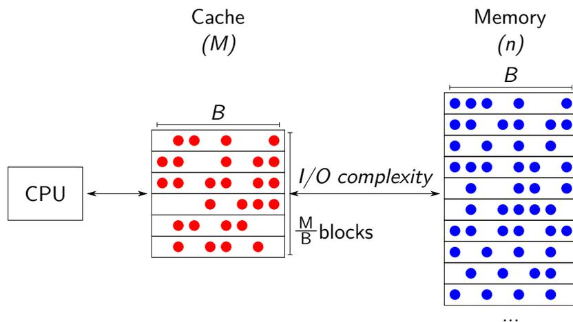
Figure 6: External Memory model with two levels of memory: the second level slow memory on the right of size  $n$  and the infinitely fast first level memory on the left of size  $M$ . Memory transfers are done in blocks of size  $B$ .
