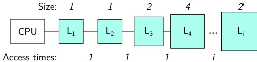
Figure 3: Hierarchical Memory Model. Memory size is growing exponentially, access times between each level is constant.
